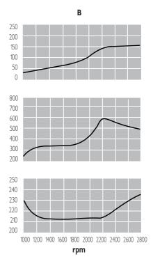
**B** = Light duty. Full throttle operation restricted within 10% of total use period. Cruising speed at engine rpm < 90% of rated speed setting - Maximum useage 1500 hours per year.
