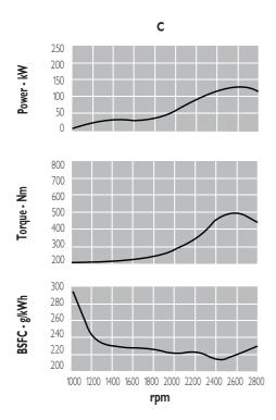
**C** = Medium duty. Full throttle operation < 25% of use period. Cruising speed at engine rpm < 90% of rated speed setting - Maximum useage 3000 hours per year.
