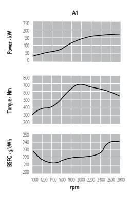
**A1** = High performance crafts. Full throttle operation restricted within 10% of total use period. Cruising speed at engine rpm < 90% of rated speed setting - Maximum useage 300 hours per year.
