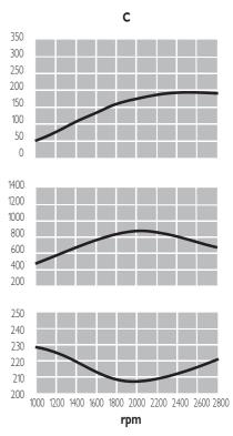
**C** = Medium duty. Full throttle operation < 25% of use period. Cruising speed at engine rpm < 90% of rated speed setting - Maximum useage 3000 hours per year.
